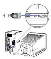
There are two ports: one for DVI screens and one for common VGA and CRT screens. Make sure you are using the appropriate connector.
